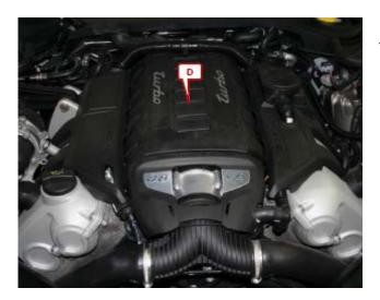
Open the engine hood. Remove the engine cover (D). The engine cover (D) is not screwed.
