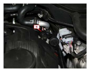
Connect the camshaft signal adapter between both connections.
